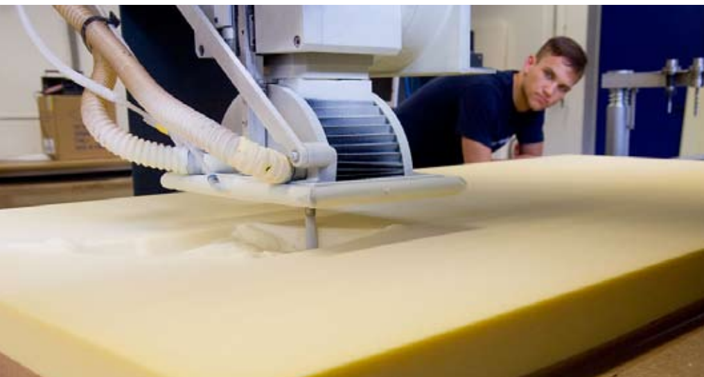
It’s up and away from Darmstadt! ROHACELL® is a material that can be perfectly shaped into the cores of sandwich components—as are used in helicopter rotor blades, for example—by using high-precision CNC technology.
